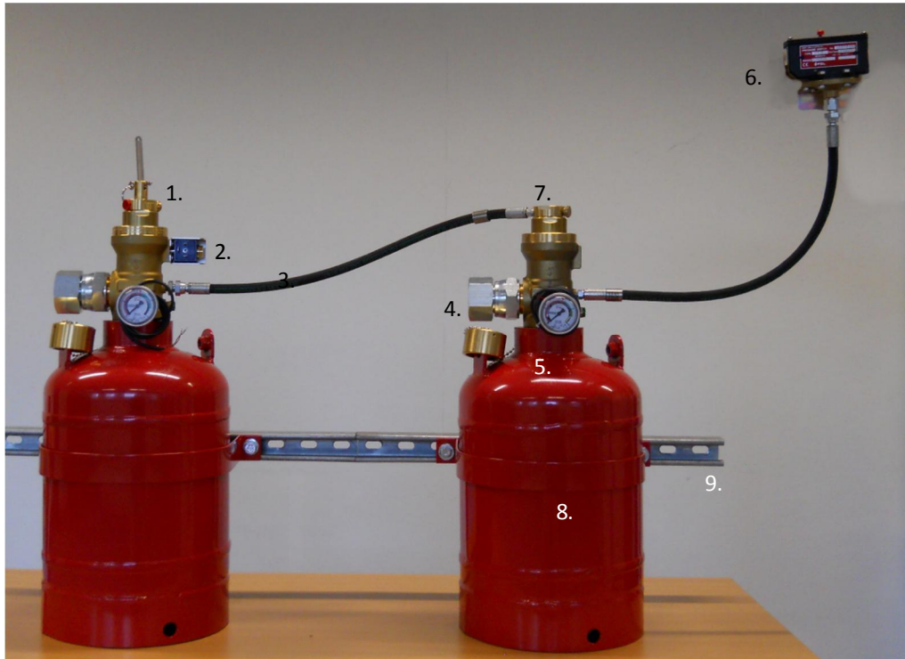
Glossary: 1. Pneumatic manual actuator 2. Integrated Solenoid 3. Actuation hose 4. Outlet adaptor 5. Cylinder Pressure gauge 6. Discharge pressure switch 7. Pneumatic actuator 8. Cylinder strap 9. Unistrut (supplied by customer)
