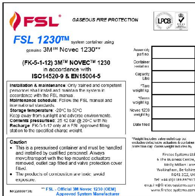
Fill label positioned on each cylinder body (part number NF22000613).
